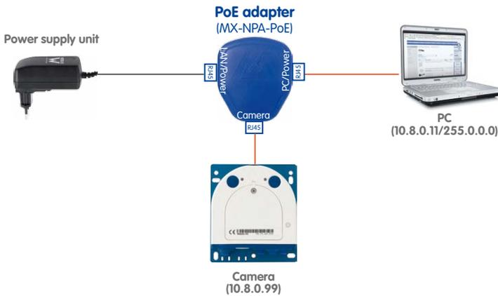
The IP addresses in the diagram are shown only as an example
