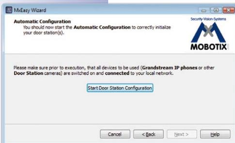
In this case, the MxEasy **Wizard** executes the auto configuration and guides you through the setup of the attached modules, the bell button profiles, etc. in a step-by-step manner.
