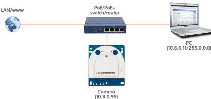
The IP addresses in the diagram are shown only as an example
