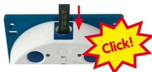
3. **Insert the MicroSD card:** Push the MicroSD card as shown (electrical contacts pointing towards the front) into the card slot using a pair of tweezers. Make sure that you hear a **click** when the card is inserted. The card is now locked and can be used. **If you are using a new MicroSD card, it needs to be formatted first** (see Section 3.5.2, «Formatting the MicroSD Card»).
