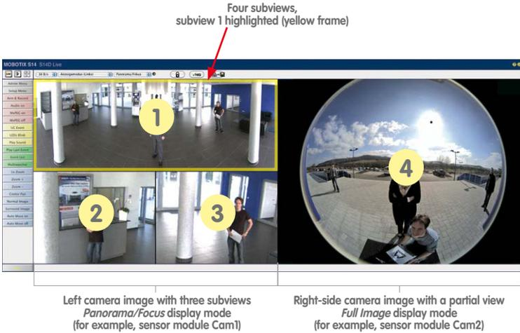
When you click inside one of the subviews, this area is highlighted with a yellow frame. All of the PTZ actions triggered by the mouse, joystick or OnScreen Control now only apply to the highlighted subview.
