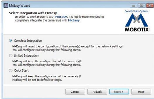
Here, you can jump directly to the main window of MxEasy with the current live camera image by activating the option **Quick Start**. However, some required detailed configurations may have to be made at a later time (for example, password protection, available bandwidth). For this reason, we recommend activating the option **Complete integration** and complete the remaining dialog boxes of the MxEasy Assistant until the main window appears.
