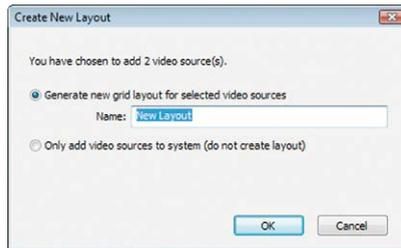
The **Create new layout** dialog box is displayed. If you select the **Generate new grid for selected video sources** option here, MxControlCenter automatically generates a grid layout that displays windows of the same size for all selected video sources. Give each layout a unique name (for example, *Underground garage*).
