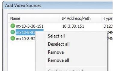
If you have cancelled the camera configuration process or need a password that differs from the camera's factory default password, you can also configure the camera from the shortcut menu at a later date and enter the user name and password required for reconfiguration at that time.
