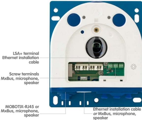
Before laying the Ethernet installation cable, remove the bayonet catch and replace the Ethernet patch cable plug with either one of the additional plugs (M.4/5) or the single wire plug (2.10), depending on the cable used.
