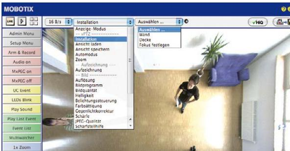
When you are setting up a S15D with two sensor modules, specify their mounting positions separately in the **Installation (right)** and **Installation (left)** Quick Control fields for the right and left sensor modules (i.e., camera images) respectively.
