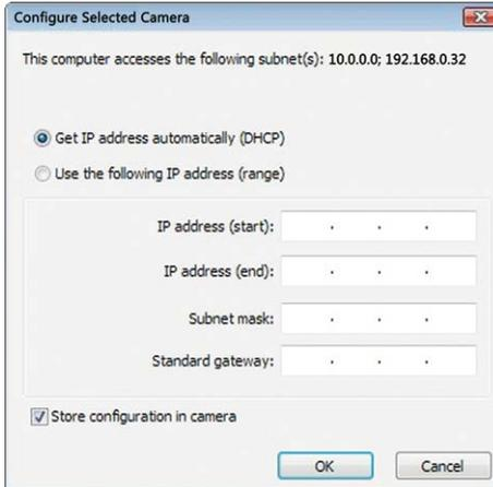
Make sure that the **Store configuration in the camera** checkbox is selected. This setting ensures that the cameras are displayed with the correct network settings even after they have been rebooted. Click **OK** to close the dialog box.
