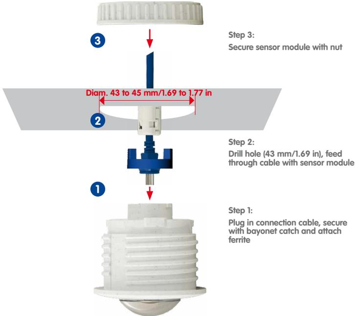
It should be ensured when selecting installation sites that each of the sensor cables do not exceed 2 m/6.6 ft. The theoretical maximum distance between the two sensor modules of a S15D where the base module is placed centrally is therefore 4 m/13.1 ft.
