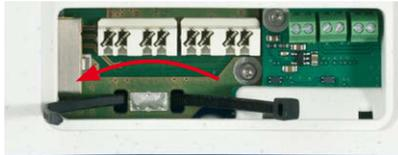
3. **Prepare the installation cable:** Cut the installation cable to length, feed through the white single wire plug (5-7 mm/0.2 to 0.28 in), remove 35 mm/1.38 in of insulation and separate into individual twisted wire pairs including 15 mm/0.6 in sheathing. Wind the shield mesh around the sheath to a width of 10 mm/0.4 in so that it can be fixed on the contact surface later using the cable tie.
