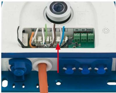
5. **Connecting the cable wires:** The individual wires of the installation cable can be connected to the LSA cutting clamp using an appropriate tool and in accordance with the EIA/TIA-568A or B standard used (see printed color coding above the clamp; see red arrow in the illustration below).
