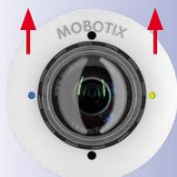
Make sure **MOBOTIX** lettering is pointing upwards!
