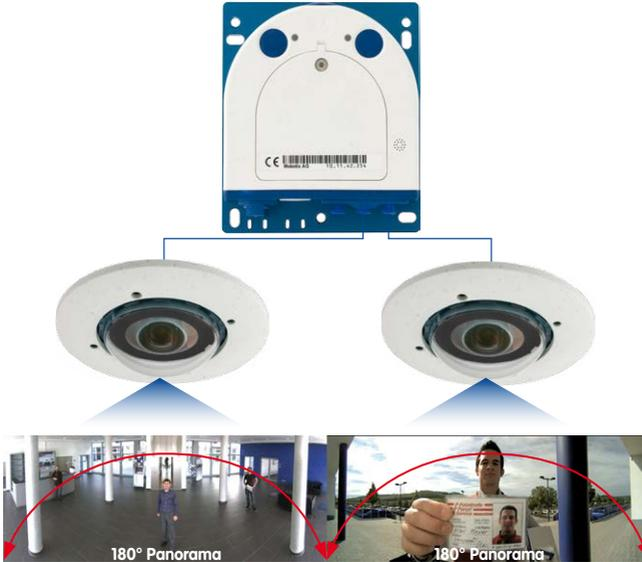
**S15M – Camera with Hemispheric Sensor Module for Concealed
