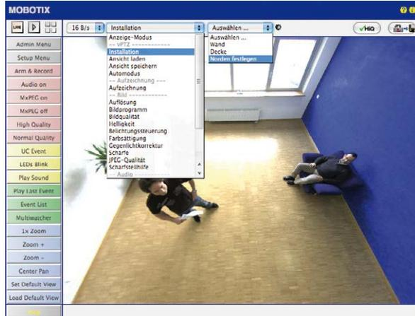
4. Store the desired North direction permanently by first activating the checkbox and then clicking on **Yes**.
