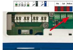
The terminal connector has two connectors to connect an MxBus module (other MxBus modules can then be connected from there). The length of the entire MxBus cable may not exceed 50 m/55 yd.
