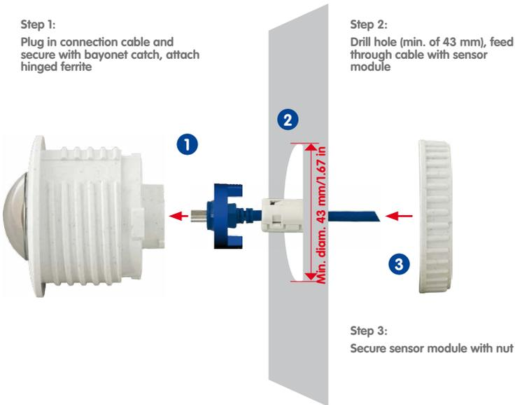
Sensor modules can be replaced any time
