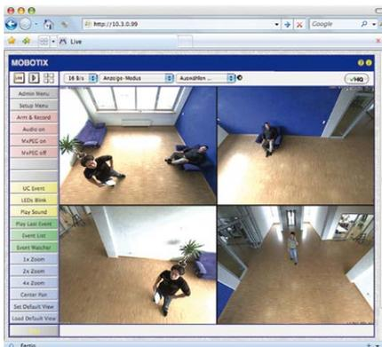
open the camera's Quick Installation in the browser's user interface. This is where you can configure the desired network parameters of the camera. Once you have completed the Quick Installation, you can connect the camera with its new network parameters to the desired network.
