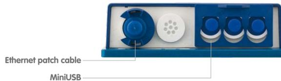
Cables with straight plugs can be used for the S15 on the camera only
