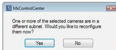
A DHCP server automatically assigns IP addresses for network devices in most networks so that you can automatically select the default setting **Get IP address automatically (DHCP)** in the **Configure selected cameras** dialog box.
