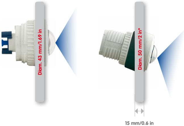
MOBOTIX also offers the appropriate installation accessories for mounting the sensor module on thicker walls. Longer "tunnel holes" through a wall can also be bridged using several extension pieces (each approx. 40 mm/1.6 in). The maximum wall thickness is therefore only limited by the length of the sensor cable depending on the installation position of the base module, which is in theory 2 m/6.6 ft.
