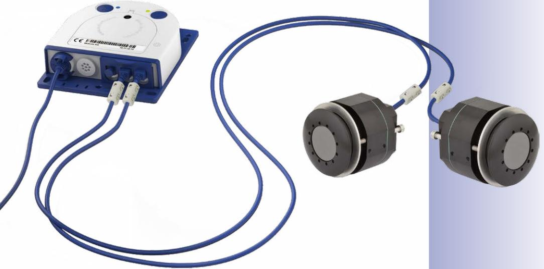
MOBOTIX S15D with 1 MX-SM-Thermal, 1 MX-SM-D12
