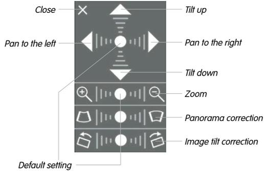
Depending on the mounting position (ceiling, wall, floor), panorama correction and mounting error correction may not be available!
