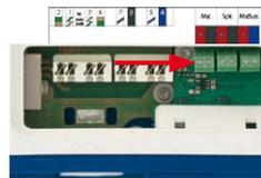
An external microphone (red box) and an external speaker (red box) with the following technical data can be connected on the terminal connector:
